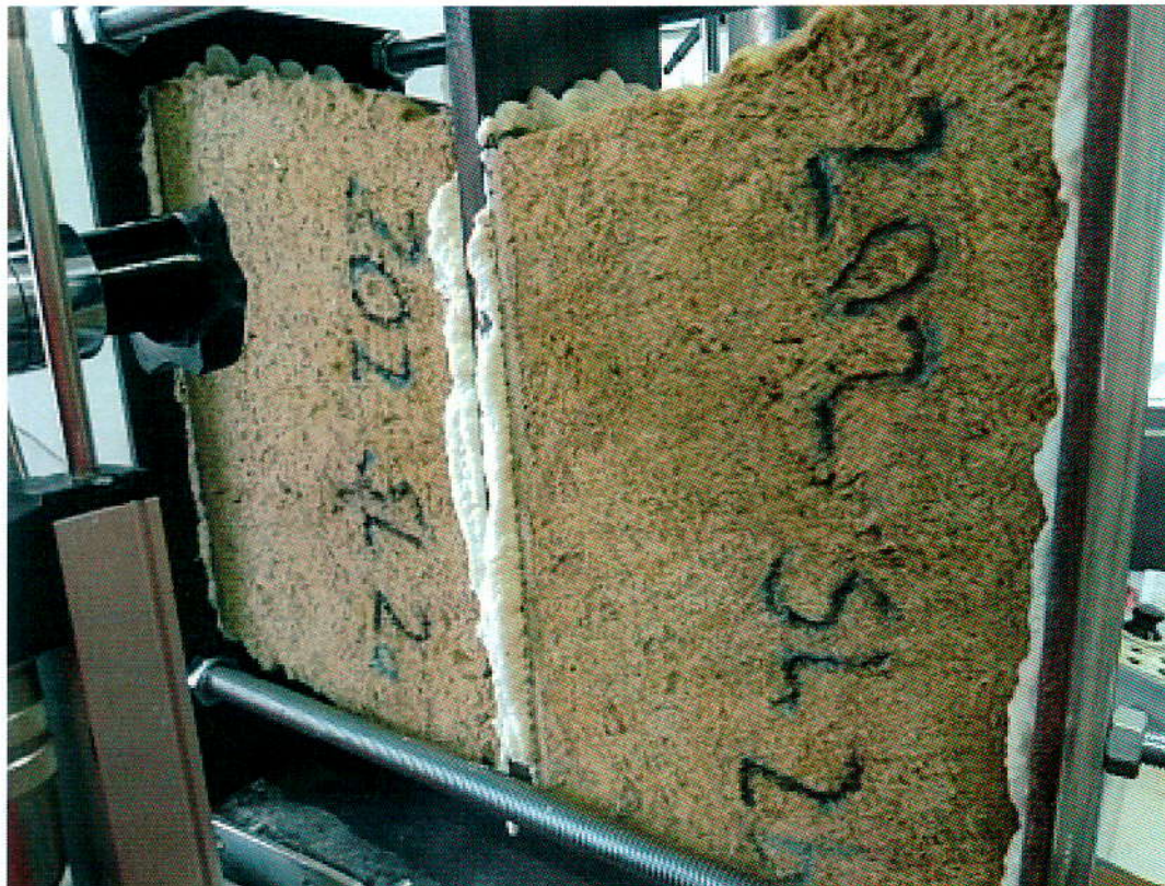
202/16 A - SHEAR BEHAVIOUR TRANSVERSE AFTER CYCLING WET SL2 - 4.0 / 232 kPa
