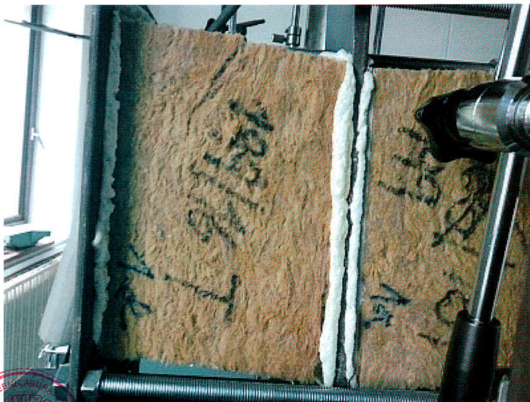
199/16 A - SHEAR BEHAVIOUR LENGTHWISE AFTER CYCLING DRY ST1 - 8.7 / 444 kPa
