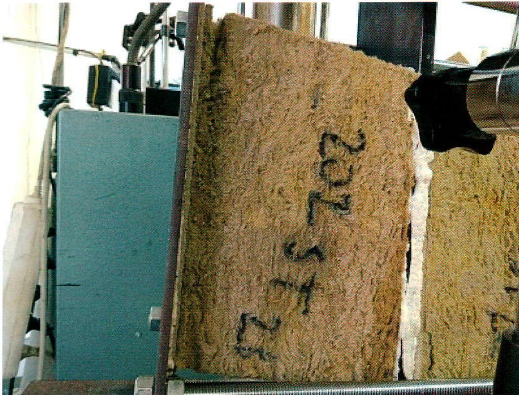
202/16 A - SHEAR BEHAVIOUR LENGTHWISE AFTER CYCLING WET ST2 - 5.0 / 409 kPa
