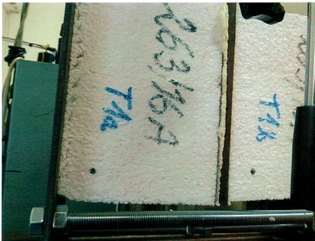
263/16 C - SHEAR BEHAVIOUR LENGHWISEREFERENCE ST2 - 41.6 / 1047 kPa
