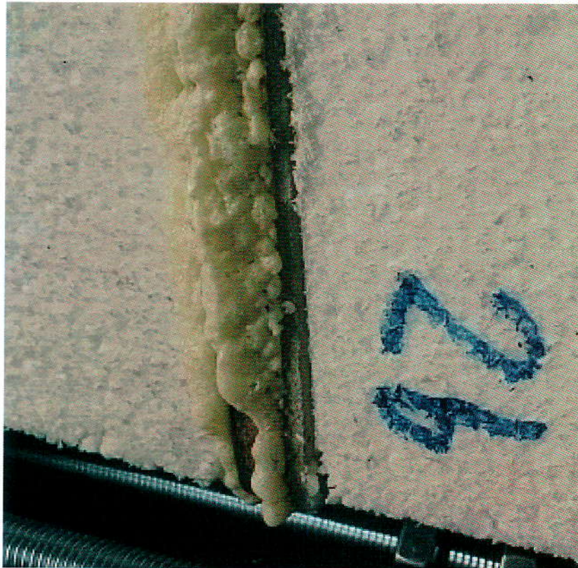
262/16 A - SHEAR BEHAVIOUR TRANSVERSE REFERENCE SL2 - 30.3 / 1003 kPa
