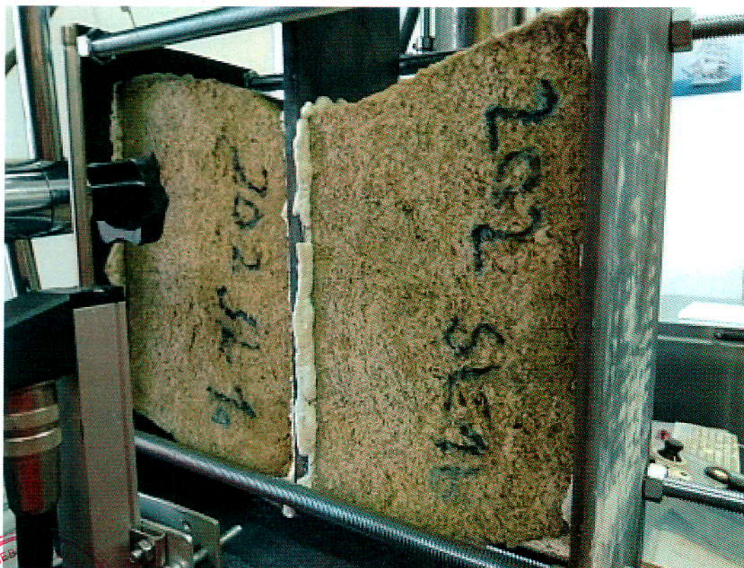
202/16 A - SHEAR BEHAVIOUR TRANSVERSE AFTER CYCLING WET SL1 - 2.8 / 226 kPa
