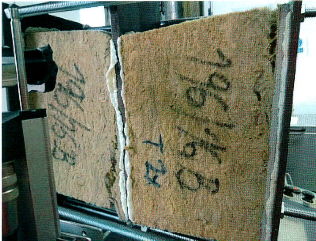
196/16 B - SHEAR BEHAVIOUR LENGHWISEREERENCE ST2 - 18.9 / 814 kPa
