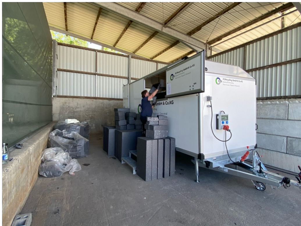
Figure 5. Mobile EPS compactor in use (source: IVH, EUMEPS, NEPSA and EPS-branchen).
