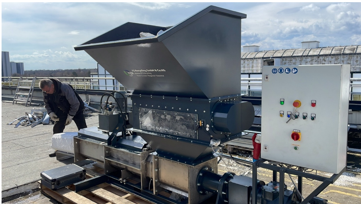
Figure 6A. Densification for recycling (source: IVH, EUMEPS, NEPSA and EPS-branchen).
